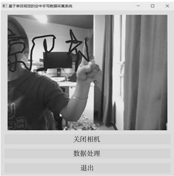
图 15 基于单目视觉的空中手写数据采集系统界面 Fig.15 Interface of in-air handwriting data acquisition system based on monocular vision
