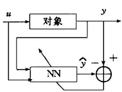
因此  $\hat{y}(k+1) = \text{NN}[y(k), y(k-1), \dots, y(k-l+1), u(k), u(k-1), \dots, u(k-m+1)]$  完成了对系统的辨识.
